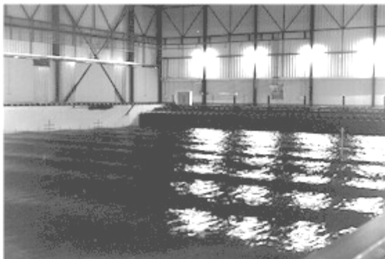
Figure 2: Generation of Waves in the Basin
