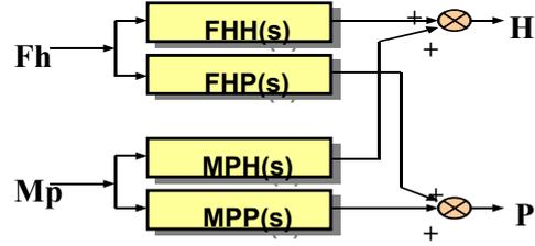
Figure 16: Decomposition of "Forces-to-Ship"
