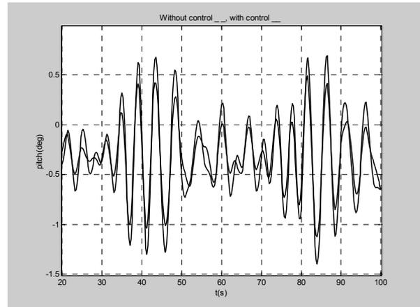
Figure 20: Effect of control on pitching.
