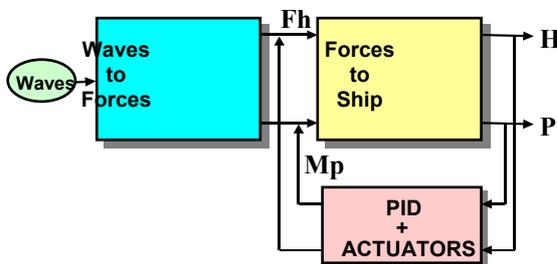
Figure 19: Diagram of the ship under PID control
