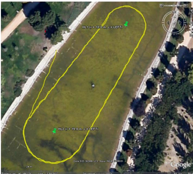
Fig. 9. GPS trace of an individual navigation control experiment along a specified Dubins path.
