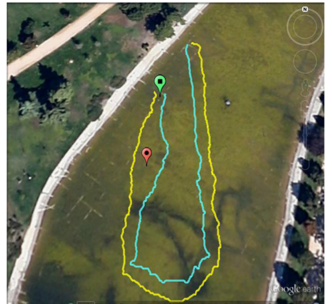
Fig. 24. Experimental confirmation of the automatic operation planning, GPS traces.
